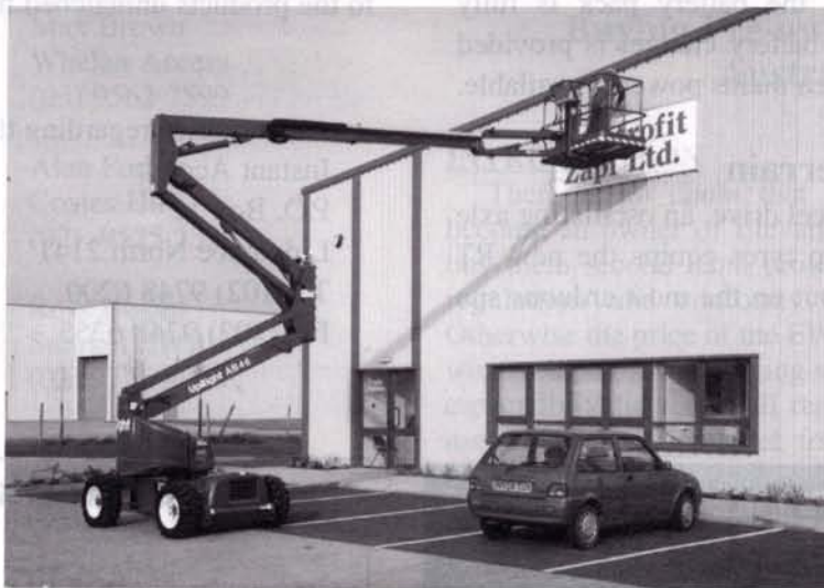
Just launched, one of the two new versions of the UpRight AB46 16m Self-Propelled Articulated Boom: the AB46 Bi-Energy version and the AB46RT (Rough Terrain) version with 4-Wheel Drive
